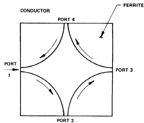
FIG. 4 FOUR-PORT CIRCULATOR USING THE EDGE-
