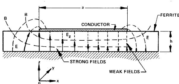
FIG. 1 MICROSTRIP LINE SHOWING RF FIELDS OF THE DOMINANT MODE.
